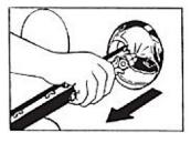
**Step 3:** Remove the bag using the pullcord or pliers.
