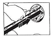
**Step 1:** Simply deflate the bag by piercing it with a screwdriver or other rigid edged tool. Make sure you do not damage the cable.
