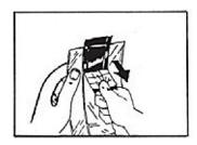
**Step 2:** Remove the protective paper of the inner sealing tape that will be in contact with the cables while unrolling the product.
